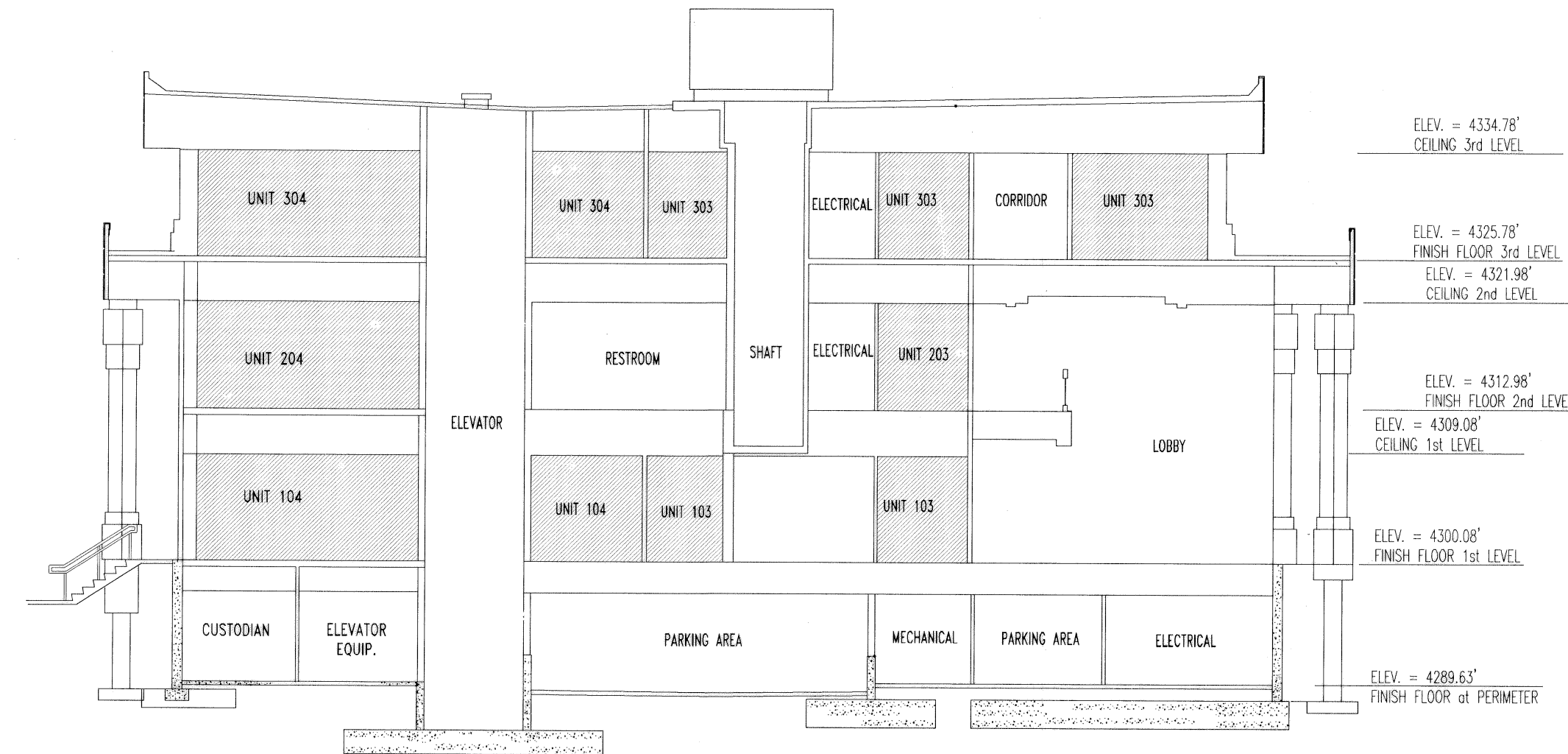
BUILDING CROSS SECTION B
