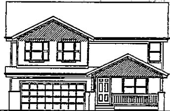
**Gable End Area** - The Gable End Area shall include areas above the eave soffit and below the rake soffit.
