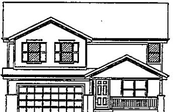
**Fenestration Area** - The Fenestration Area shall include the rough opening area of windows and glass area of doors. Garage door windows shall not be included (a value of zero shall not be accepted).
