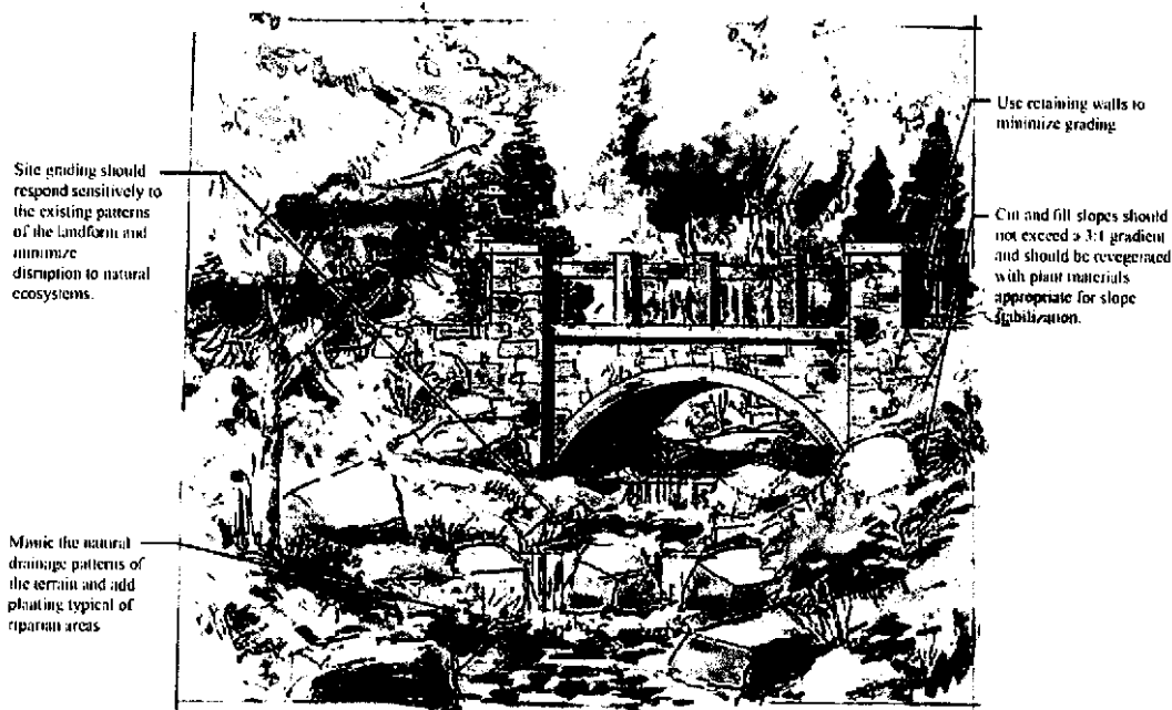
Figure 8: Grading and Drainage
