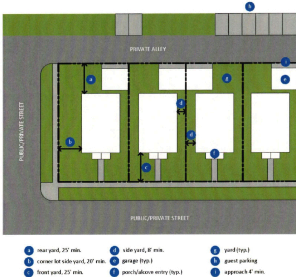
Figure 2 Sample patio home layout diagram with detached garage located in rear of lot with direct alley access.
