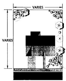
TO RETAIN 32 C-FT ON EACH LOT PER LID ASSESSMENT, PLACEMENT AND METHOD OF RETENTION IS UP TO OWNERS DISCRETION
