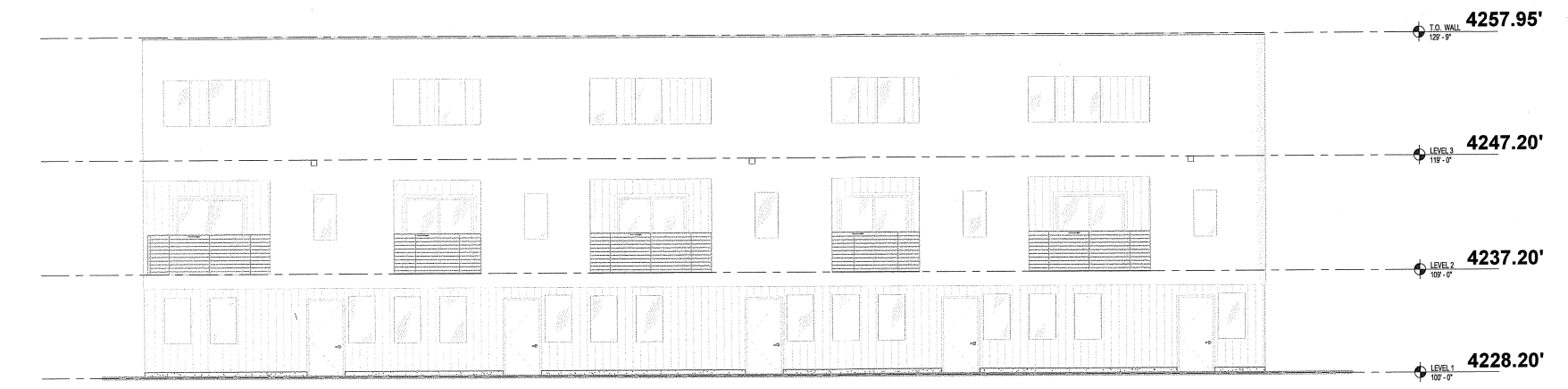
4 BUILDING - C: ENTRY ELEVATION Scale: 1" = 10'
