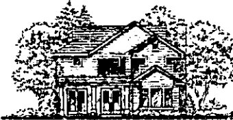
Side-to-side gables One and two story massing
