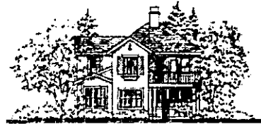
Varied rear-facing slope with some intersecting hip elements Added porch and balcony
