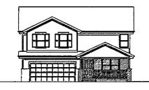
Porch/Deck Area - The Porch/Deck Area shall include all areas of an elevation perpendicular to the line of sight covered beneath the horizontal surface of the porch or deck. All surface areas counted shall not be recounted in another category (e.g., fenestration or masonry piers falling under a porch roof).
