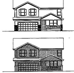
Surface Area - The Surface Area shall include all wall areas of an elevation perpendicular to the line of sight, including gable end area, porch/deck area, fenestration area, and masonry area, but shall not include fascia.
