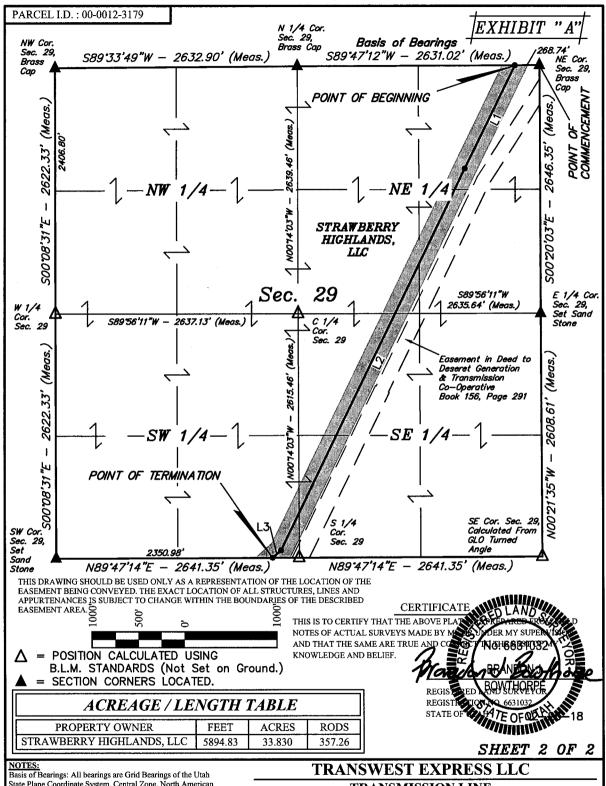
Basis of Bearings: All bearings are Grid Bearings of the Utah State Plane Coordinate System, Central Zone, North American Datum 1983 Based on GPS Observation of the Monuments Shown Hereon. All Measured Distances Shown are Ground Distances
